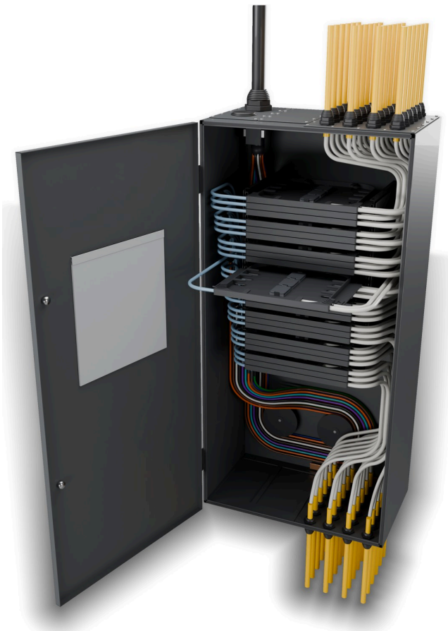
48 x 144F build: 24 exits through the top feed trays 1-12, 24 through the bottom feed trays 13-24. Tray 10 slid out.
