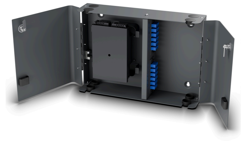
Doors open. 2x 12-port SC/UPC plates on the center partition; black metallic splice trays and radius guides on the left. Pigtails not pictured.
