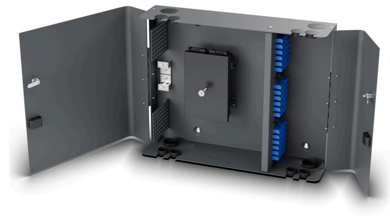
Doors open. Ribbon LC build, 144F: 6x 24-port LC/UPC plates and black metallic splice trays. Pigtails not pictured.
